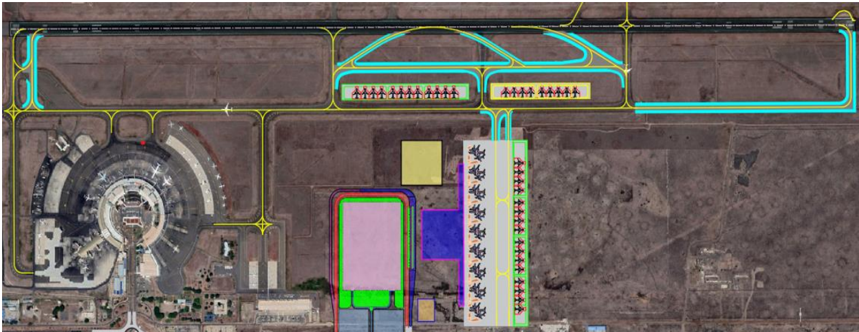
Figure 73: Phase 3 Taxiway Development Works – Extension of PTT and Link Taxiways and Apron
