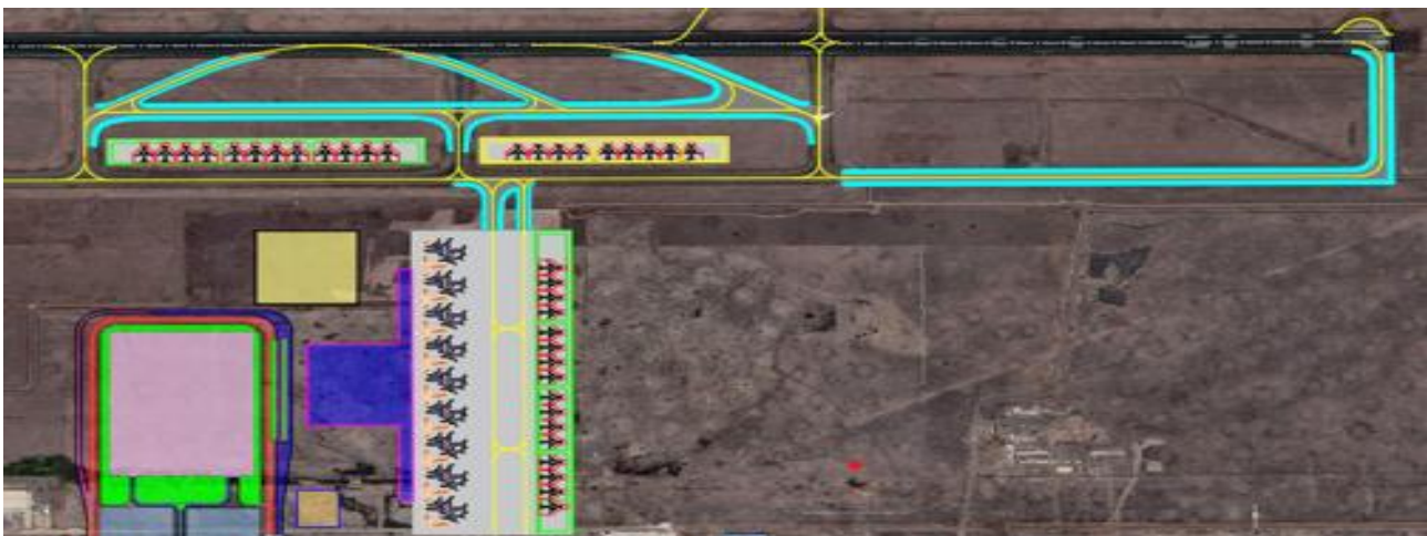
Figure 76: Phase 3 Commercial Apron Development Works – Contact & Remote Stands
